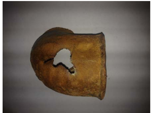
Picture 8 Galvanized pipe inside the building
